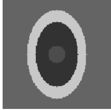
Fig. 1. Simulated phantom used for the investigation. The object consists of a background region with \bar{D} = 100 \mu\text{m} , an outer cortical ring with \bar{D} = 200 \mu\text{m} , an inner medullary ring with \bar{D} = 50 \mu\text{m} , and a central circular region with \bar{D} = 75 \mu\text{m} .
