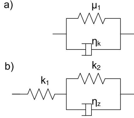
Fig. 3. In the upper half of the figure, a), Kelvin-Voigt model is diagramed. Model consists of a elastic component  $\mu_1$  in parallel with the viscous component  $\eta_k$ . In the lower half of the figure, b), we illustrated a standard linear solid or Zener model, which is represented by a series of an elastic component and a Kelvin-Voigt model.
