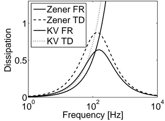
Fig. 5. Dissipation factor as a function of frequency for the Kelvin-Voigt and Zener models for fresh and thermally-damaged porcine liver.
