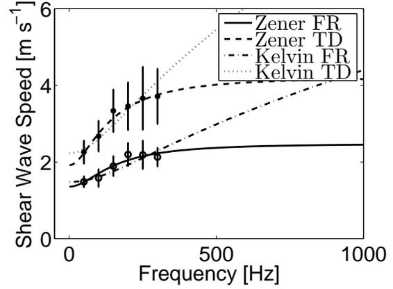
Fig. 4. Comparison of the shear wave speeds as a function of frequency for the Kelvin-Voigt model and the Zener model for both fresh and thermally-damaged porcine liver.
