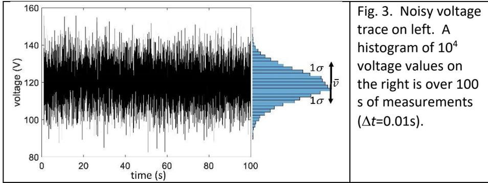
Fig. 3. Noisy voltage trace on left. A histogram of  $10^4$  voltage values on the right is over 100 s of measurements ( $\Delta t=0.01s$ ).
